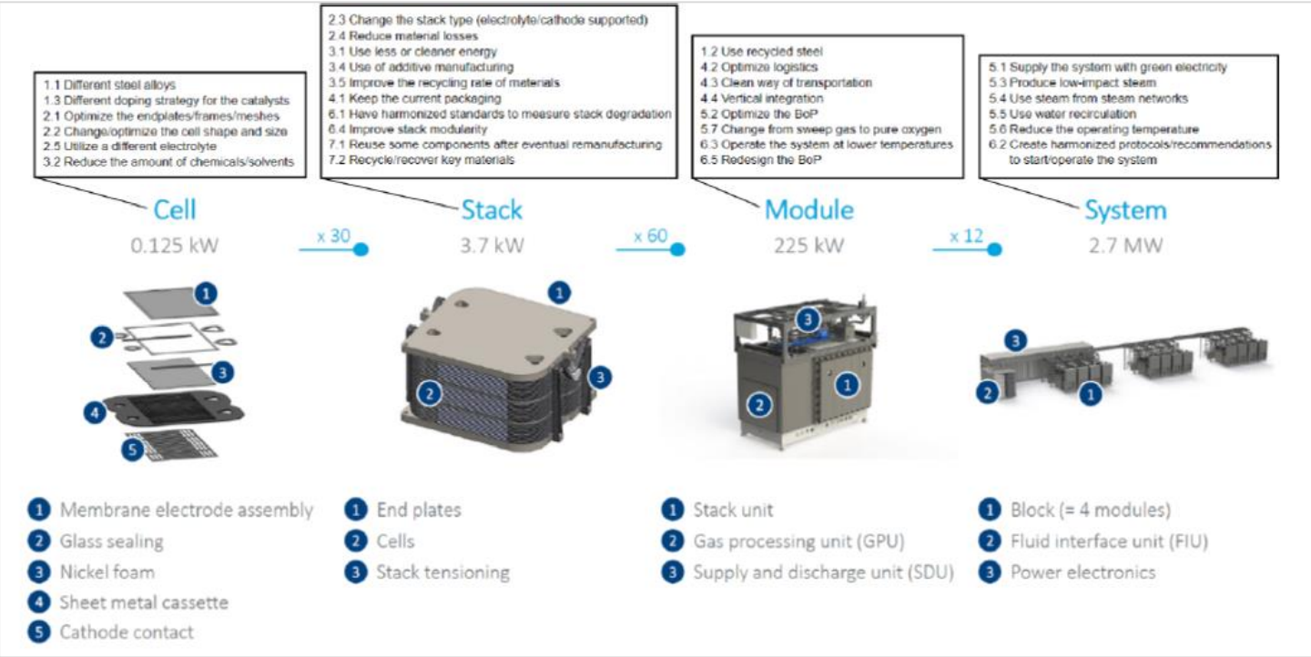
Schematic of the solid oxide system and eco-design actions in developing product concepts (original image courtesy of Sunfire GmbH) [eGHOST D3.2]
